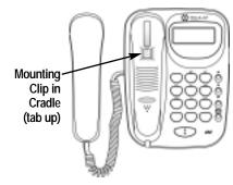
Figure 11 – Handset mounting clip assembly.
